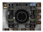
IOP readings, average values and corrected IOP are all clearly displayed on one screen.
